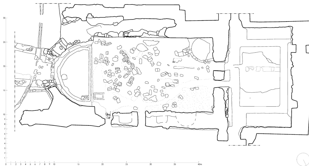
Fig. 10 – Salamis central calidarium, Terrestrial Digital Photogrammetric survey plan (Copyright: Camiz, Tedeschi, Griffo 2018).
