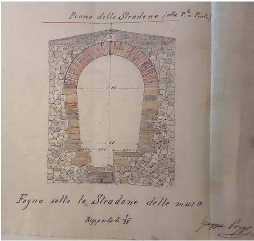
Fig. 11 - Original sewer section from Giuseppe Poggi's project. Sewers, different years 1866-1895 AS-CFi CF7800
