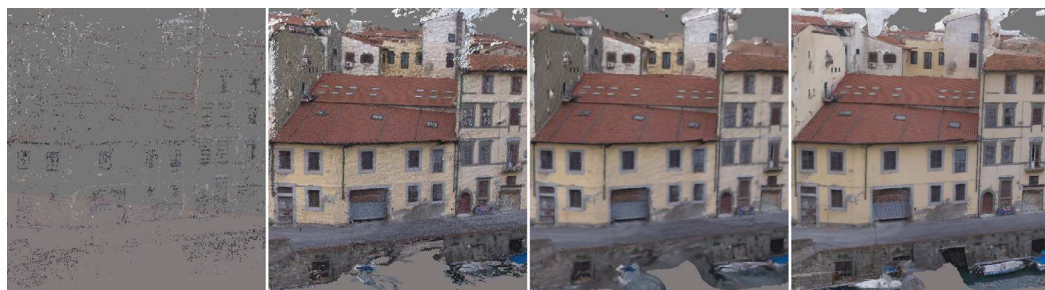
Fig. 1a, b, c, d - a) sparse point cloud, b) dense point cloud, c) mesh, d) textured mesh
