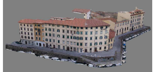
Fig. 4: textured model elaborated from the photos taken by the drone, the model looks well-proportioned and with very few parts missing.
