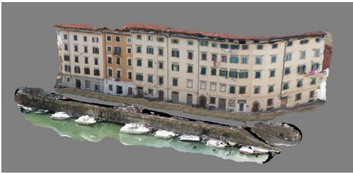
Fig. 2 - Textured model created with the photos taken from ground level, the missing parts caused by blind spots are rather evident.
