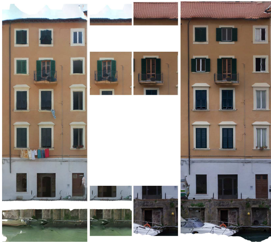
Fig. 6 - A comparison between a section of the model elaborated from photos taken from ground level (on the left) and the model elaborated from photos taken by the drone (on the right), with a focus on three details showing the differences on accuracy on the different heights.
