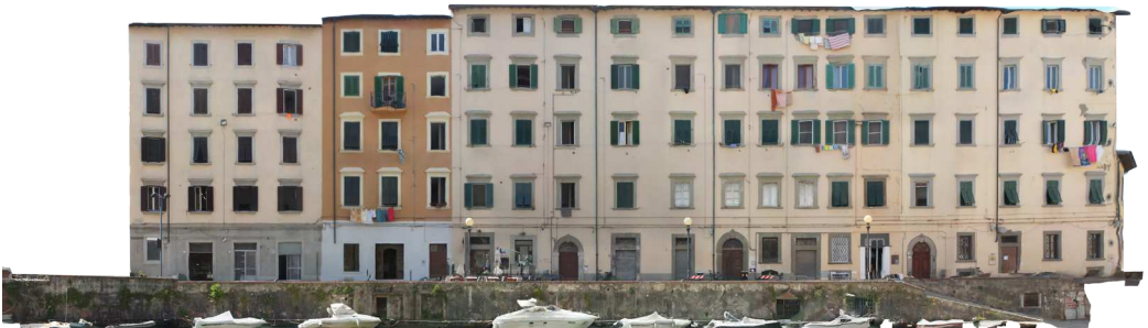
Fig. 3 - Photomap elaborated by the previous model, the roofs are missing and the upper part is quite distorted.
