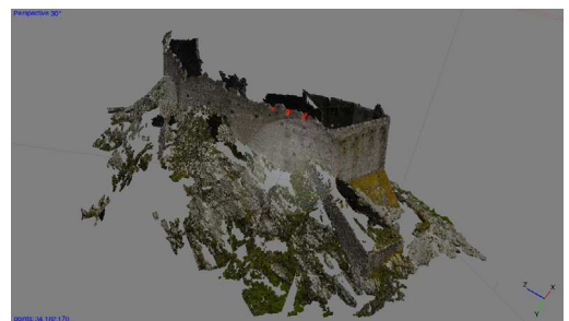
Fig. 9 – Final point-cloud generated by the alignment process. (Copyright: Mirco Pucci, Giulia Baldi)
