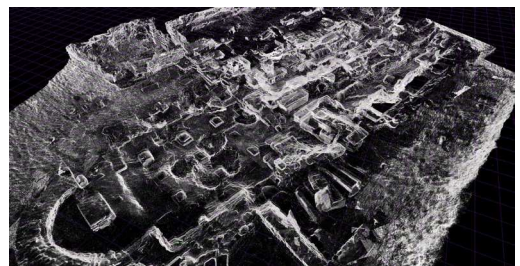
Figure 13 – 3D Laser Scanner pointcloud (aligned).
