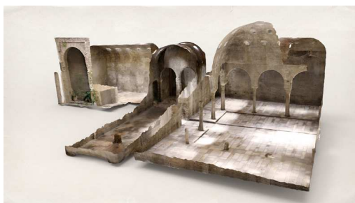
Figure 9 - Photogrammetry generated mesh with the texture coming from the shots automatically applied.
