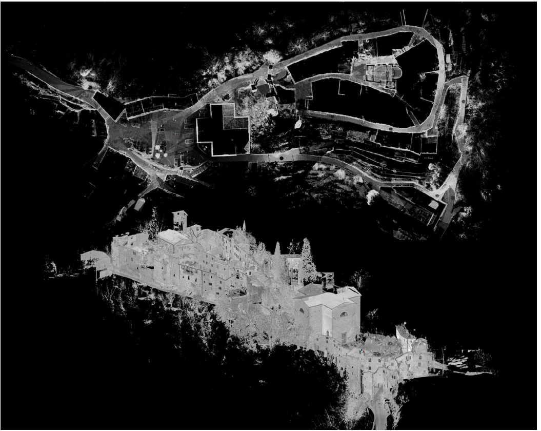
Fig. 5 – Snapshot of the point cloud made with a 3D laser scanner Faro 8080
