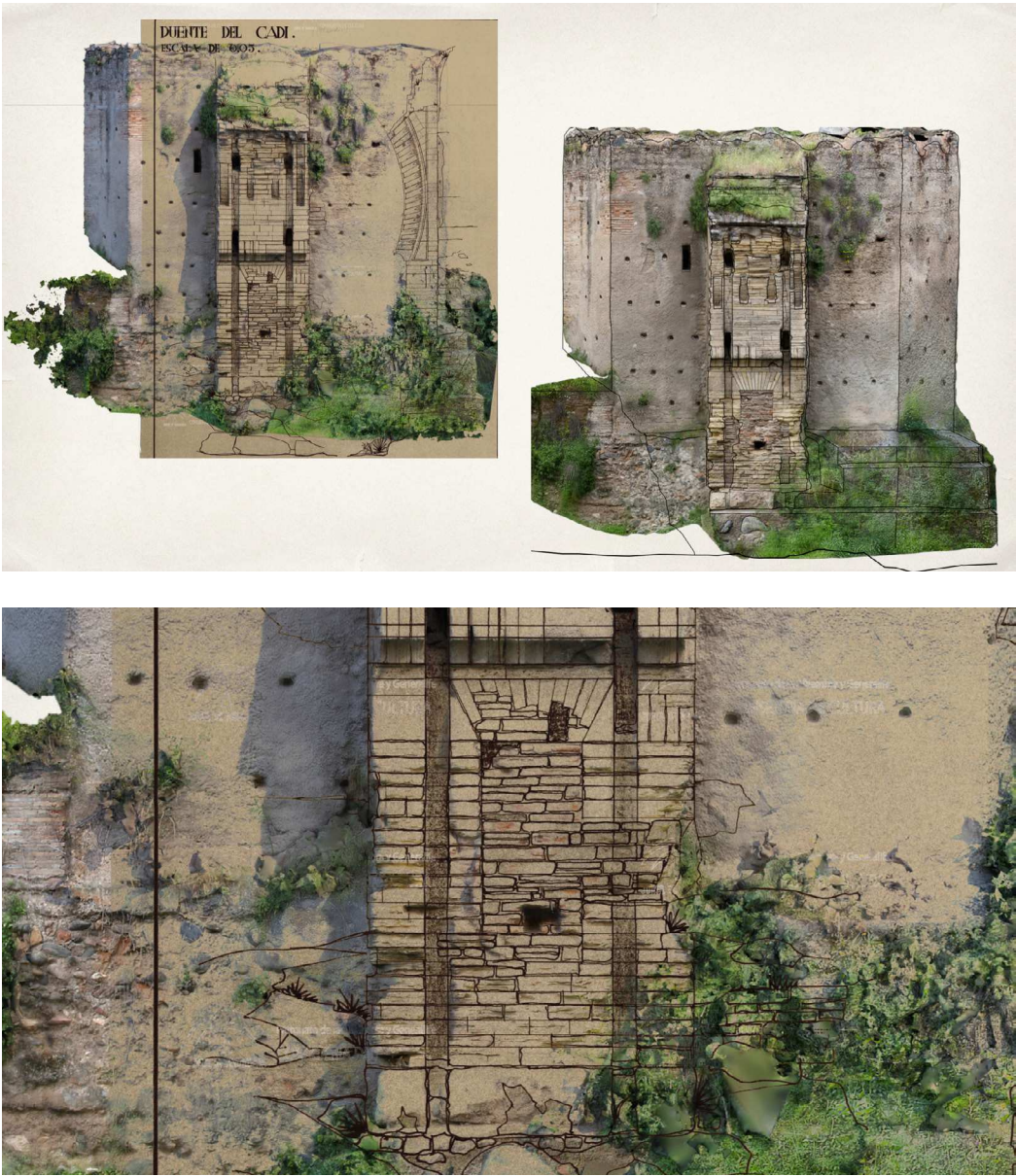
Fig.14 and Fig. 15 – Comparing the previous traditional surveys available in the Alhambra archives with the new digital survey.
